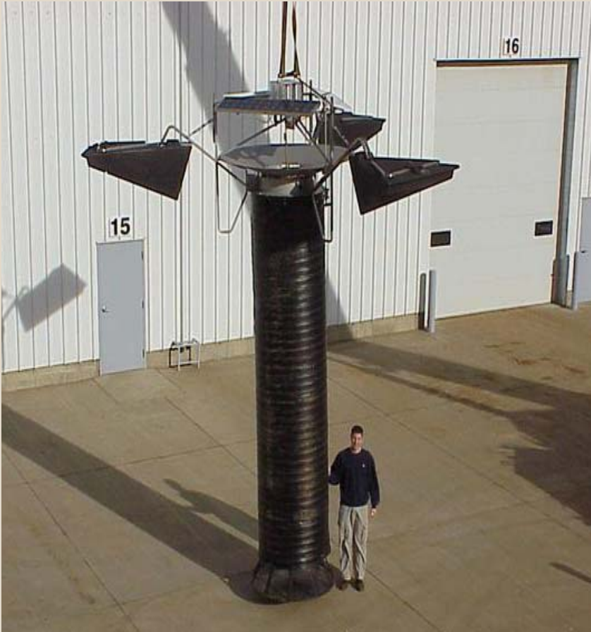
SolarBee - Lake Mixing Apparatus for climate change experiments
